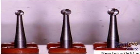
New burs (left) and damaged burs after repeated usage and sterilization (right)
